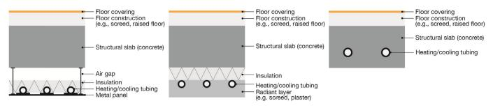
Fig. 1. Illustration of radiant panels (left), embedded surface systems (ESS) (center) and thermally activated building systems (TABS) (right).
